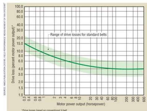
FIGURE 5. Belt loss. Higher belt speeds tend to have greater losses than lower belt speeds at the same horsepower.
