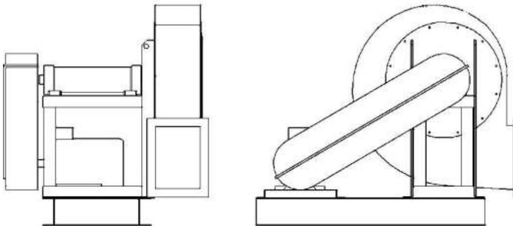
Belt driven centrifugal fan (Arrangement 12 )
