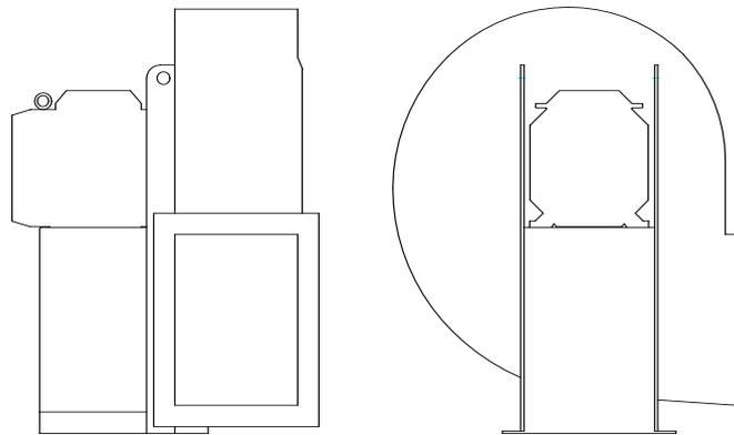
Direct driven centrifugal fan (Arrangement 4 )
