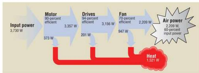
FIGURE 6. Energy loss in a typical fan.
